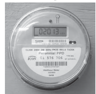
New residential AMI meter
